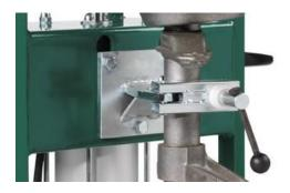
To <u>make sure</u> that the lips on both spring holders are <u>correctly seated</u>, <u>pull the swivel arms outward</u> by slowly building up down-pressure. *If the spring holders can be pulled out, the lips are not clamping properly!!*
