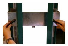
This prevents lateral movement of the spring holder arm. When you have finished replacing the shock-absorbers do not release the lock at the rear of the balance cantilever until you have released the pressure on the spring.
