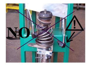
Use the press for pressing springs on McPherson struts only!
