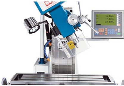
Swiveling cutter head with sliding quill
