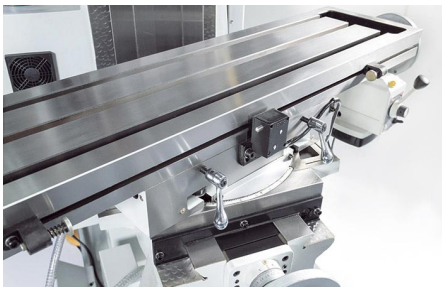
Cutter table swivels in X axis
