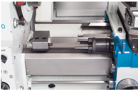
Central lubrication is integrated into the support for easy maintenance and handling
