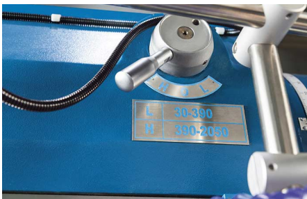
Powerful headstock drive with auxiliary gearbox (Servomill® UWF 12)
