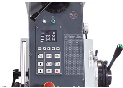
Spindle speed, depth stop, and quill position are shown on the display
