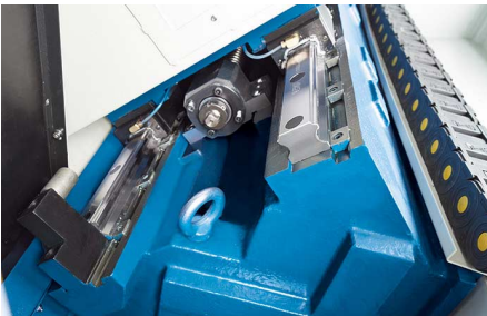
45° inclined bed with linear guides
