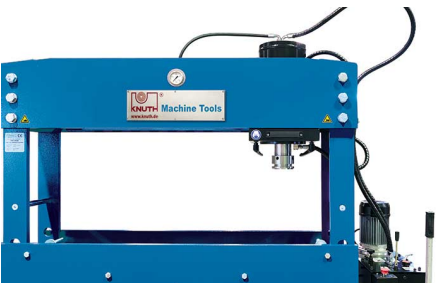
The hydraulic cylinder can be moved laterally and is clamped mechanically
