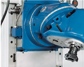
2 swivel levels allowing to set virtually any angle
