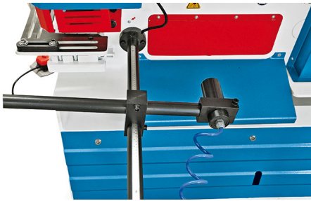
Back gauge with automatic cut activation
