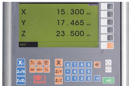
Positioning indicator on X, Z and Z1 axis
